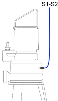
If you have any internal seal probe, it will have leads in one of the pump cables. In order to determine which internal seal probe is installed, check whether or not the pump is FM-approved explosion proof. If it is an explosion proof model, it will have “FM” at the end of the model number. If the pump is an A-Series model (AMX, AMS, AV(X), AK(X)), it is also important to determine which motor frame size the pump is. This is given by a letter D, T, P, F, G, or H in the model number.
