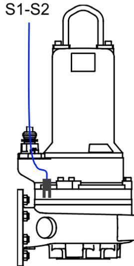
If the pump is an F, G, or H motor frame, there will be an additional dual wire seal probe in the motor cap junction chamber. This is wired as S3 & S4. The oil chamber monitor should be wired as above, depending on if the model is explosion proof.
